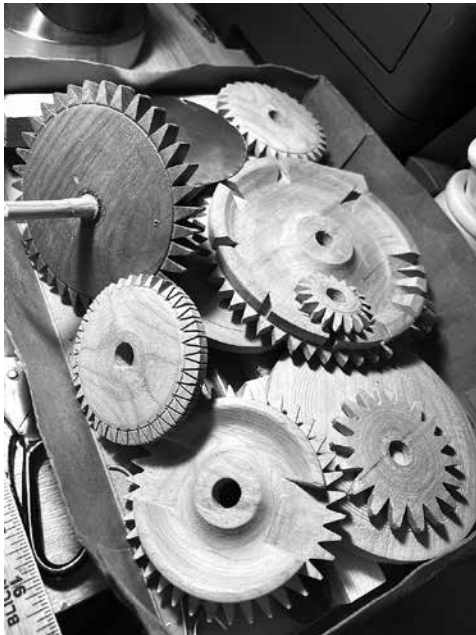
These wooden clock gears are typical of the gears used in Cheney clocks.
